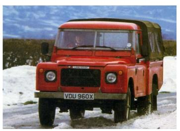
are replaced by coils (influenced by the Range Rover). The four-cylinder engines come with all-synchromesh, five-speed gearbox. Identifiable by a full-width black plastic grille and wheelarch lips fitted to house wider track suspension.
